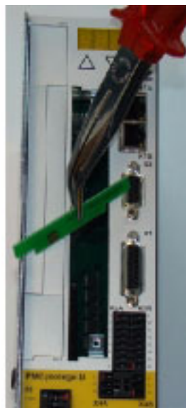
4. Using suitable pliers, pull out the blank in the safety card plug
