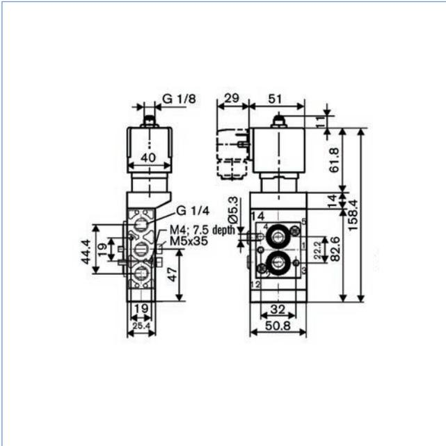
5/2-way impulse valve with NAMUR flange
