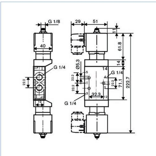
(Main dimensions of the 5/2-way model with threaded port connection and with 1 coil, see 5/2-way model with NAMUR flange)
