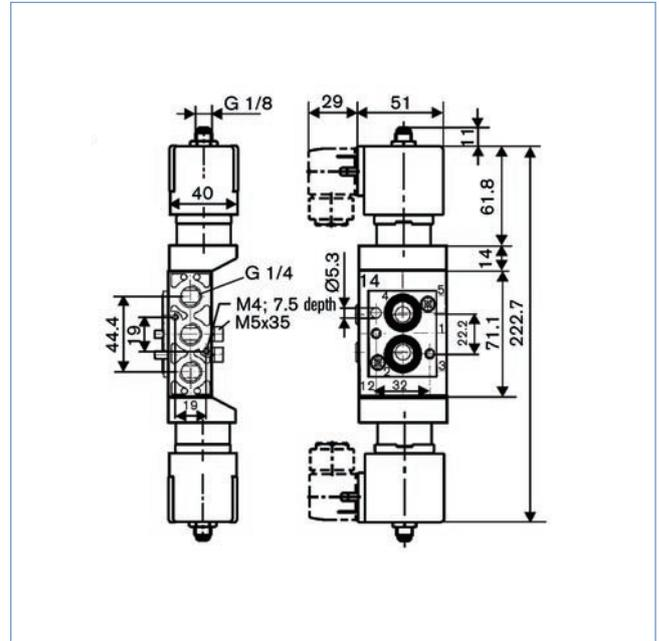
5/2-way impulse and 5/3-way valves with G 1/4 threaded port connection
